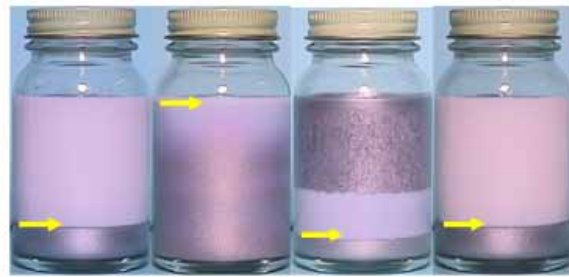
BLANK AQ-600 ASE Urethane After 30 days / R.T. / FC#4 20sec
